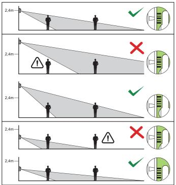
Figure 4. How the mounting height affects the detector supervised area and how the pyroelectric element should be positioned against the lens to optimize the area.
