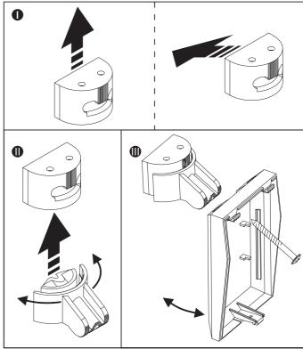
Figure 3. Mounting the detector on holder.
